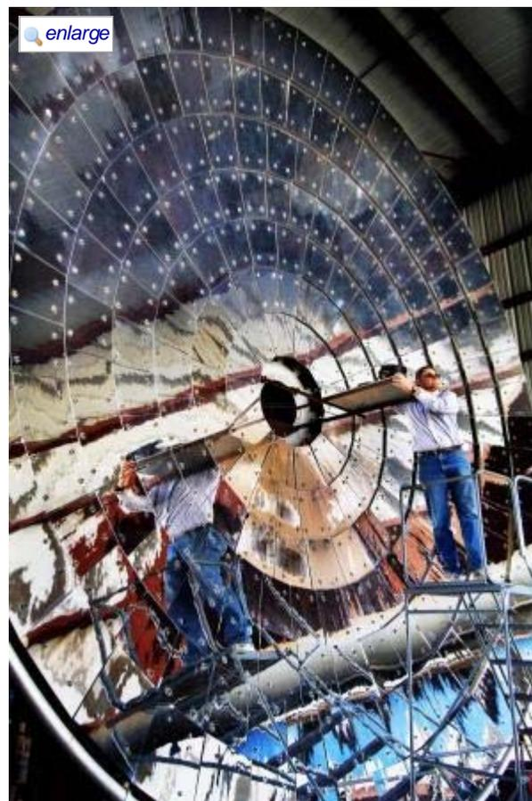
Sandia researcher Rich Diver checks out the solar furnace which will be the initial source of concentrated solar heat for the CR5 prototype. Eventually parabolic dishes will provide the thermal energy. (Credit: Photo by Randy Montoya)
