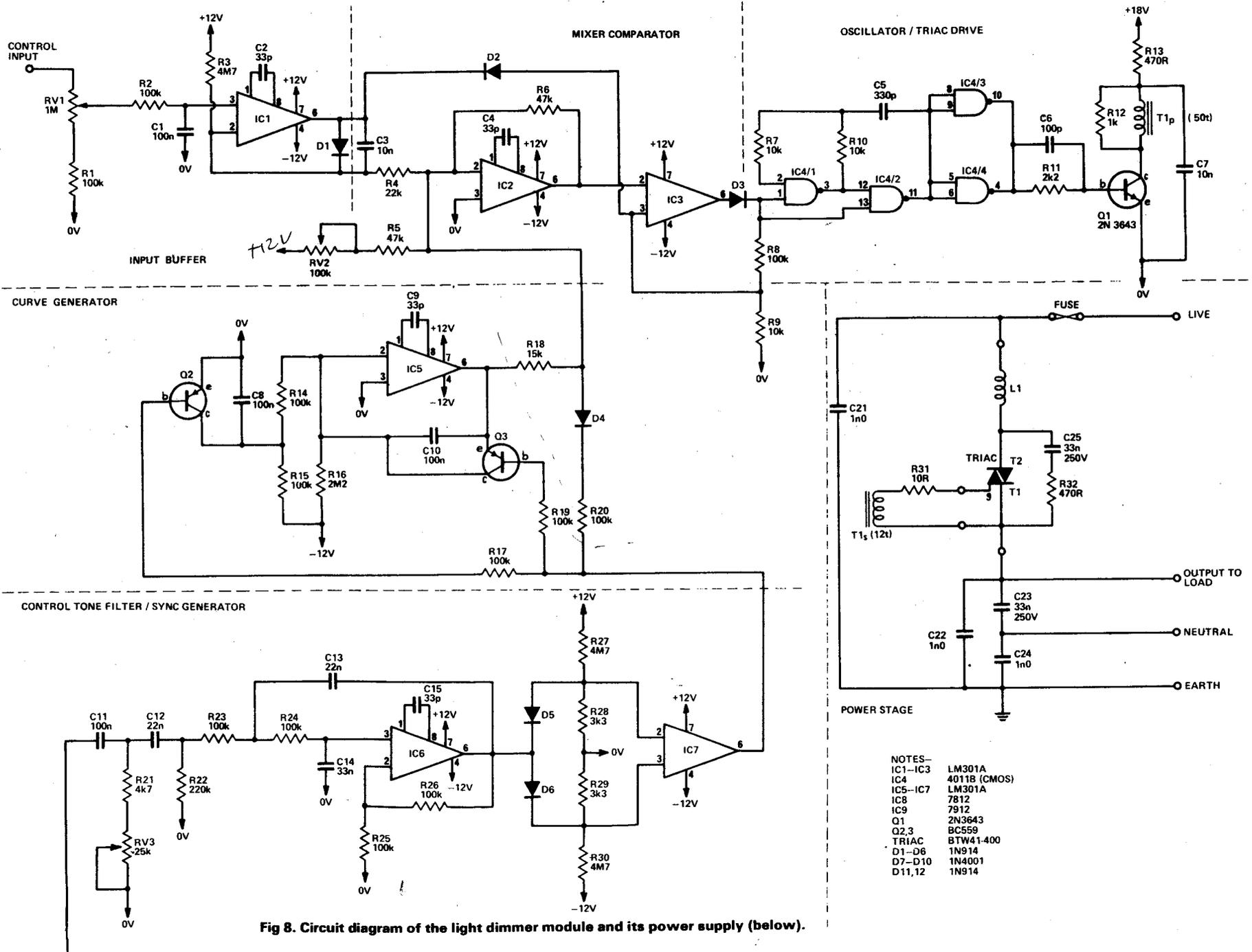
Fig 8. Circuit diagram of the light dimmer module and its power supply (below).
