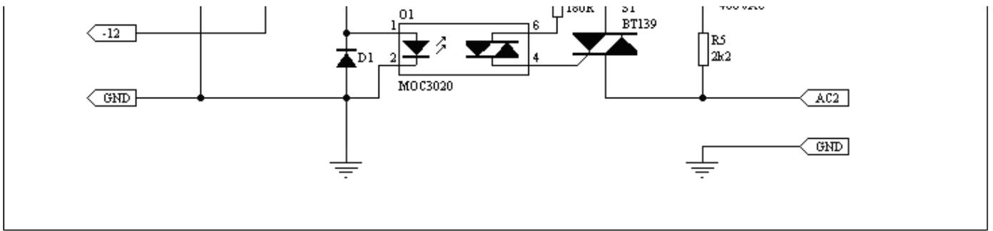
Figure 10 - Dimmer Circuit
