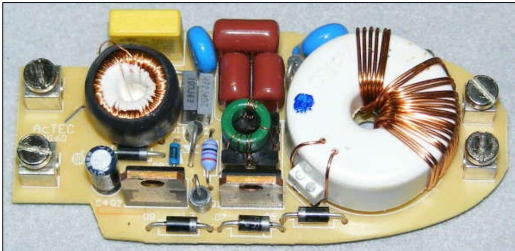
Figure 11 - Electronic Transformer Internals
