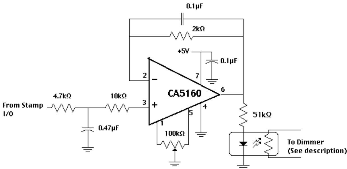
The circuit is simple, The op-amp provides current amplification allowing the optoisolator to sink current without discharging the 4.7μF capacitor. The 51kΩ resistor provides the right current through the optoisolator to provide the right resistance on the output of the optoisolator.
