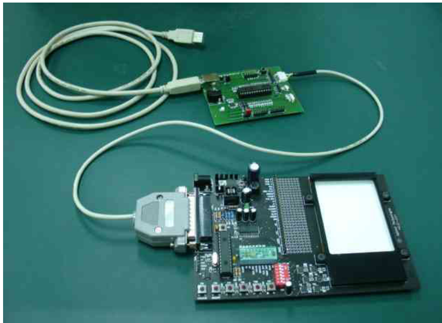
Figure 4. Setup connection for USB-2-I2C with HDJD-JD13
