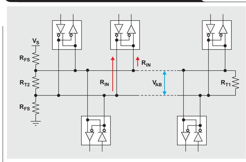
For clarity, Figure 2 shows the equivalent circuit of the RS-485 bus with the failsafe biasing resistors,  $R_{FS}$ , the terminating resistors,  $R_{T1}$  and  $R_{T2}$ , and the equivalent input resistance,  $R_{INEQ}$ , lumped together to represent the common-mode input resistance of all transceivers connected to the bus.
