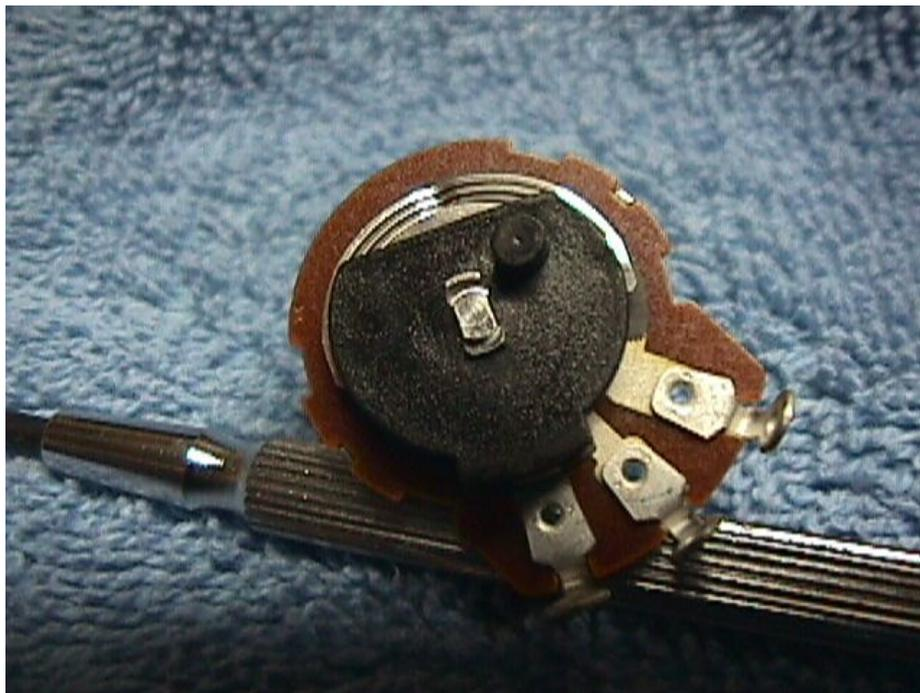
Looking closely, you can see that the shaft is held onto the plastic disk by being mechanically squashed into place. That is quick, and makes for cheap pots, but it can't be removed and successfully reassembled. That is a peculiarity of this brand, as some pots can be disassembled and reassembled successfully. In the next picture, I've used a big pair of diagonal cutters to remove the plastic disk and the metal wipers. This exposes the bare conductor assembly.
