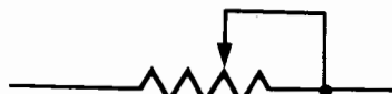
Fig. 7. Pots in some applications require only a variation in resistance. Which terminals are connected together depends on the circuit effect.
