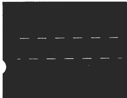
FIG. 2—THE 2N4400 TRANSISTORS have a fast rise-time; here's what the output waveform looks like.
