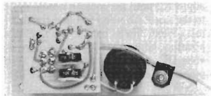
FIG. 2—THE SMALL PC BOARD can be secured to the front panel of the cabinet via S1's mounting nut. The board shown here is the author's prototype.
