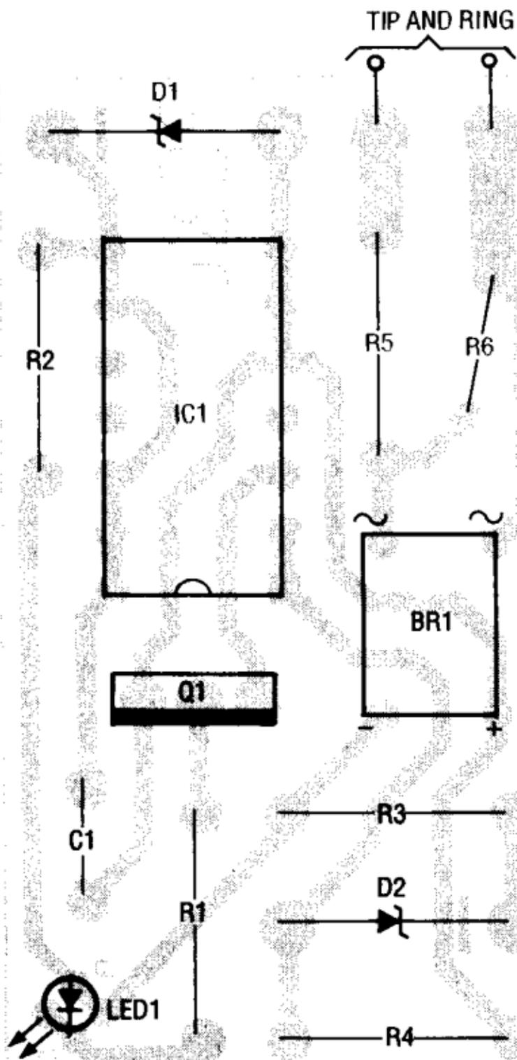
**FIG. 2—IF YOU'RE USING A PC board, follow this parts-placement diagram. The LED can be mounted so that it can be bent in any direction, or remain straight up.**
