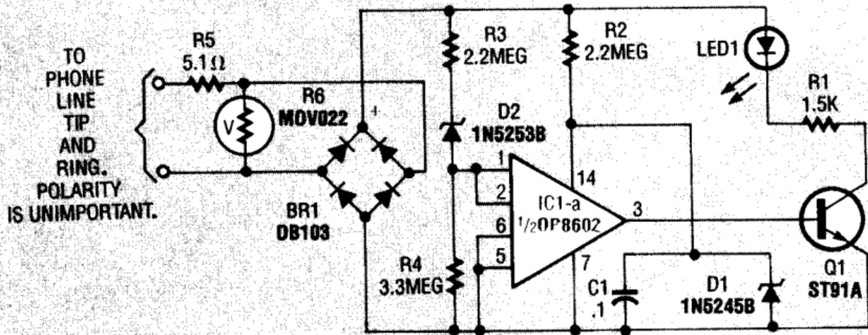
**FIG. 1—AT THE HEART** of the circuit is an ultra-low-current voltage-level sensor that draws only about  $5 \mu\text{A}$  when the phone line is not in use.
