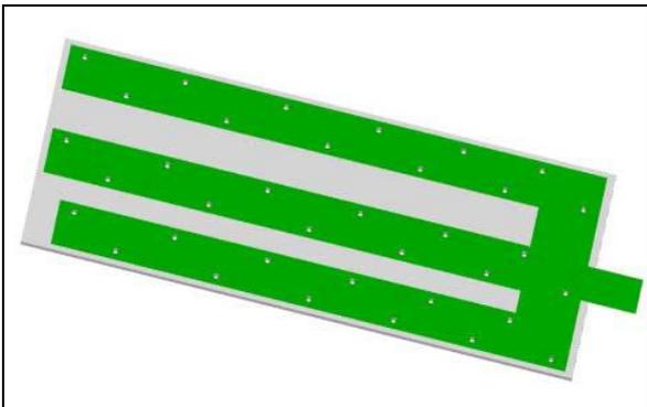
Figure 8: The flex board to be attached to the prepunched panel
