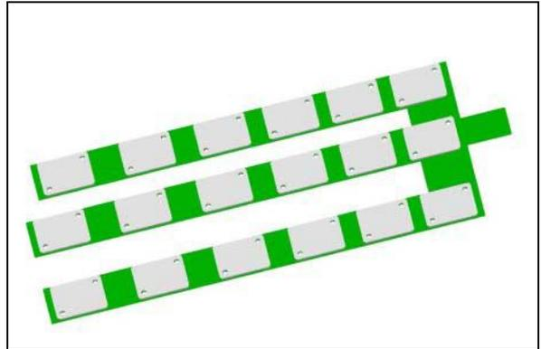
Figure 10: The backside of the punchedout flex board
