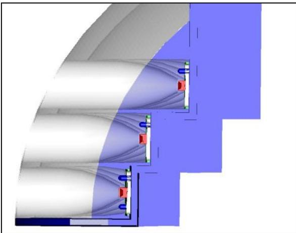
**Figure 15: The position of the LED relative to the reflector**
