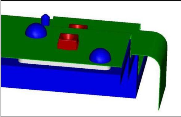
**Figure 13: Two remodeled pins which hold the LED segment in place**
