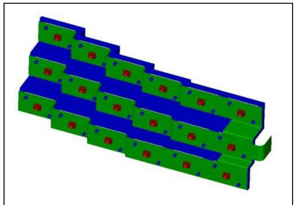
Figure 12: The assembly in which each LED segment is separately mounted on the alignment pins of the plastic carrier
