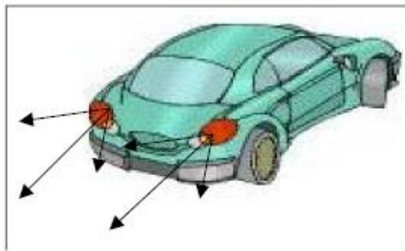
Figure 2: Emission direction of taillights
