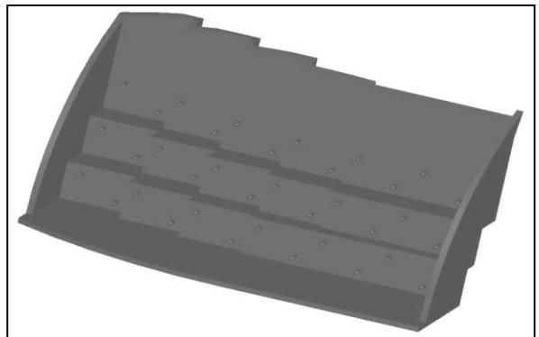
Figure 11: The plastic carrier with pins for alignment and caulking
