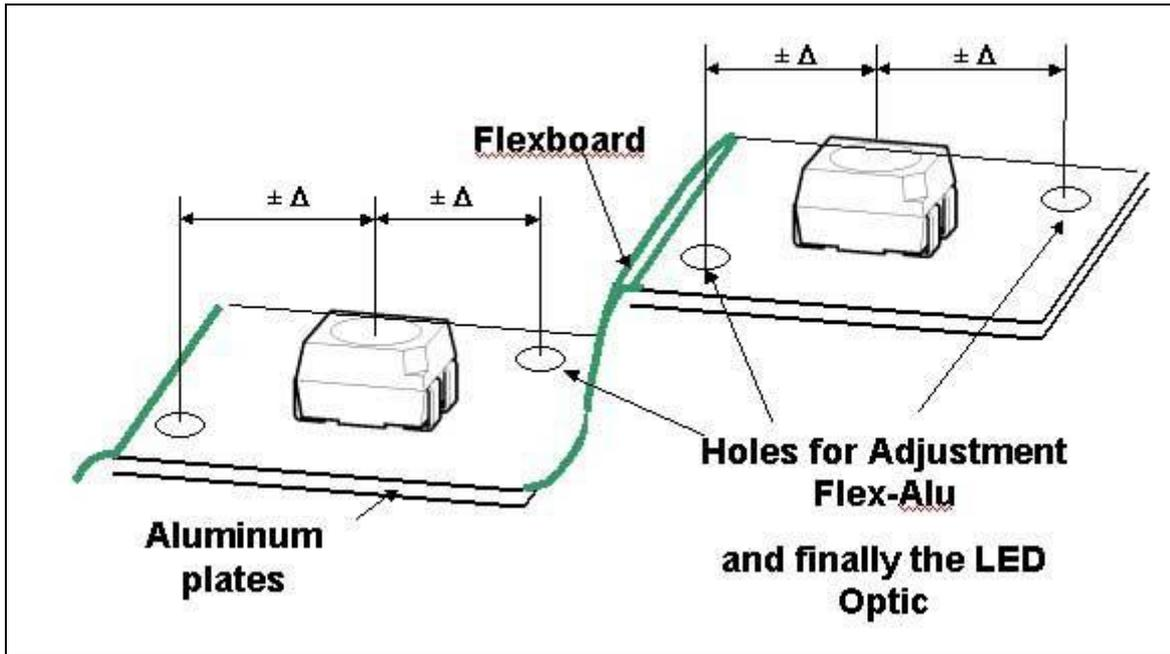
Figure 16: Schematic of tolerances
