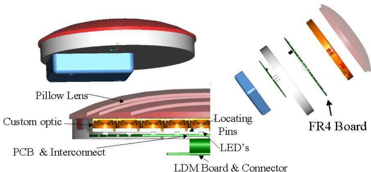
**Figure 1: 2D lamp units with SMT components on FR4 printed circuit board material**
