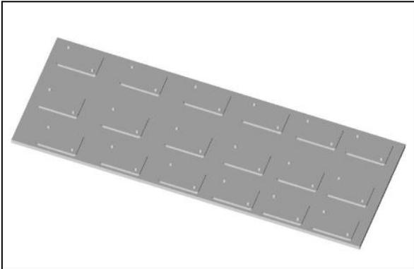
Figure 7: The prepunched aluminum panel
