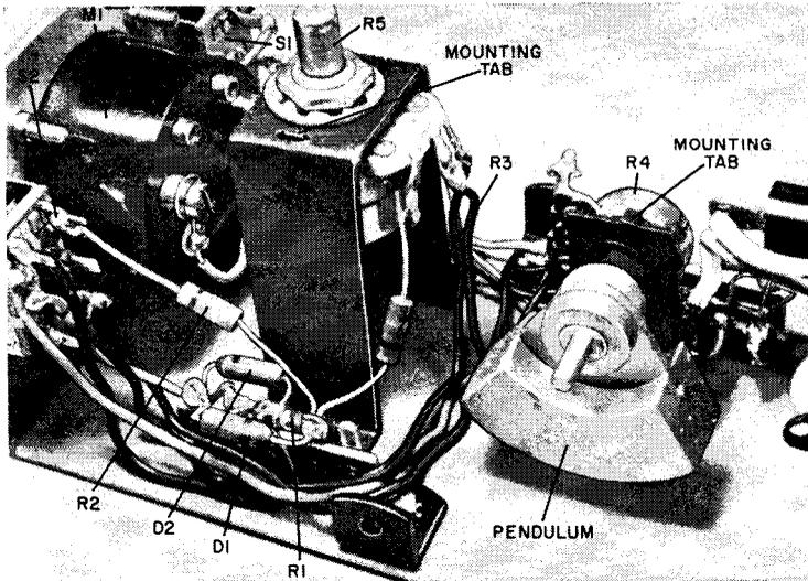
Wiring and assembly is open but very rigid. The pendulum must have room to swing freely. The shaft of zero-G setting potentiometer R5 is accessible through a hole in cover of the metal box.
