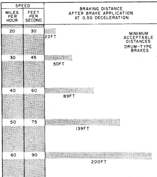
Fig. 7. The G-Whiz is an excellent device to check performance of drum or disc-type brakes. A good test is to decelerate at 0.5 G and measure the braking distance vs. miles per hour. Acceptable distances are shown in this graph. Brake fading can be observed on the G-Whiz as described in the text on page 40.
