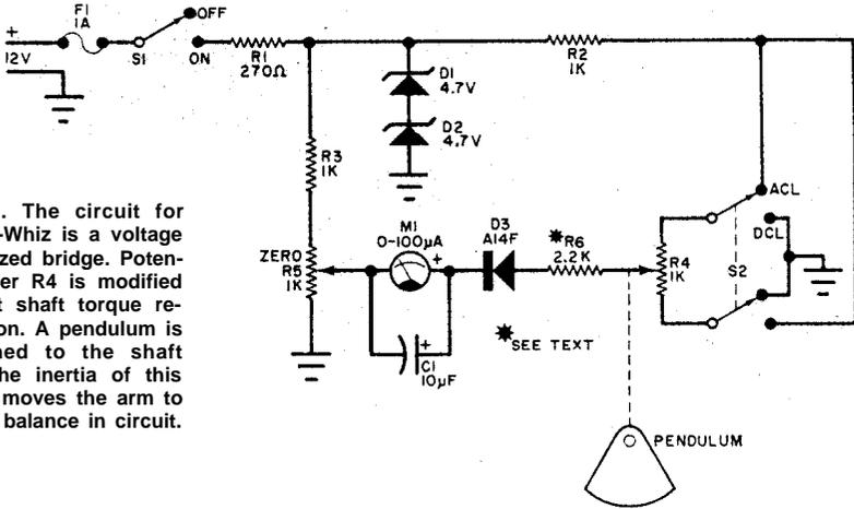
Fig. 1. The circuit for the G-Whiz is a voltage stabilized bridge. Potentiometer R4 is modified to cut shaft torque restriction. A pendulum is attached to the shaft and the inertia of this mass moves the arm to upset balance in circuit.
