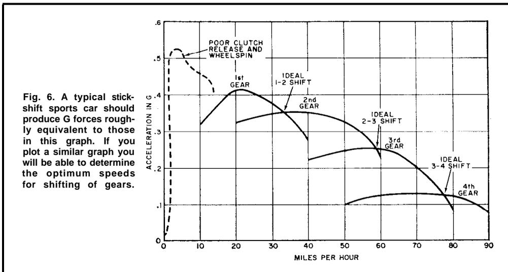
Fig. 6. A typical stick-shift sports car should produce G forces roughly equivalent to those in this graph. If you plot a similar graph you will be able to determine the optimum speeds for shifting of gears.
