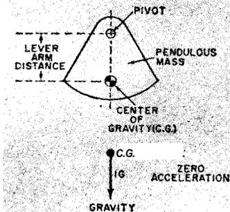
All forces acting on the pendulum mass act on its center of gravity, which is eccentric with respect to its pivot point. The lever arm is the distance from the pivot point to the center of gravity and transmits the force acting on the center of gravity to the pivot in a rotational manner.
